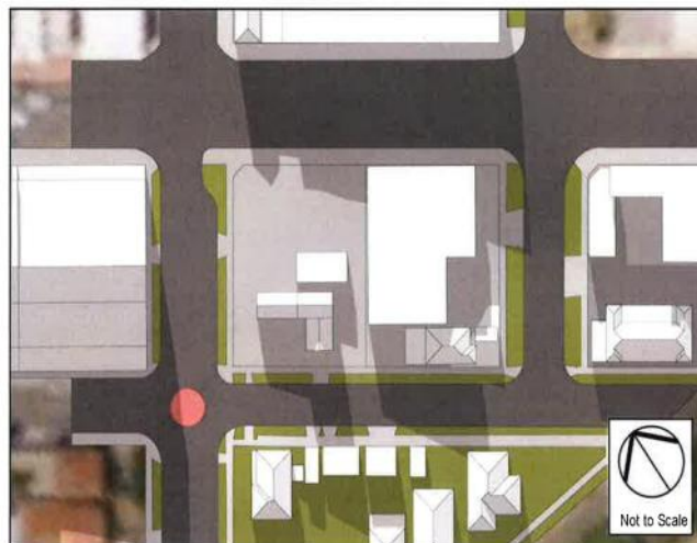
Figure 24: Existing Shadow Diagram – 9am 21 st June
