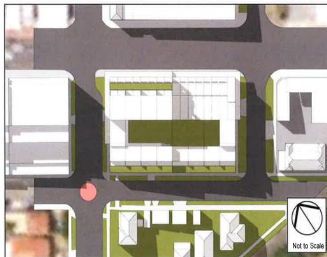
Figure 27: Proposed Shadow Diagram – 12pm 21 st June
